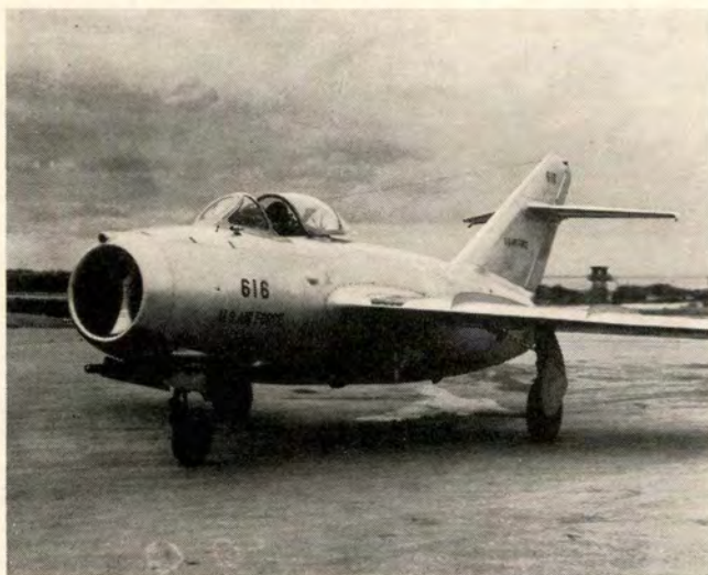
The MiG-15 was one of the first jet aircraft designed with the high-tail, swept-wing configuration to meet performance requirements. Its control characteristics often shook-up its pilots.
